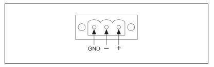
Figure 2-2. Power Receptor and Pin Assignment
